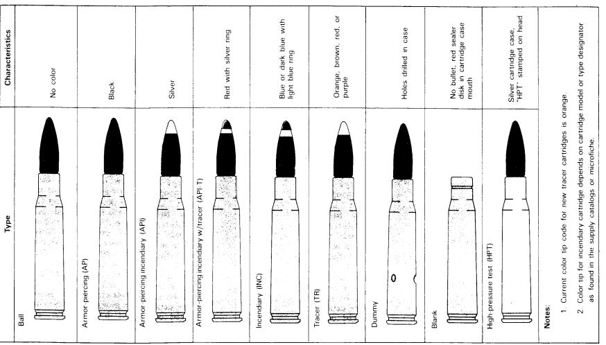
Figure D-13. Caliber .50 Cartridges.
