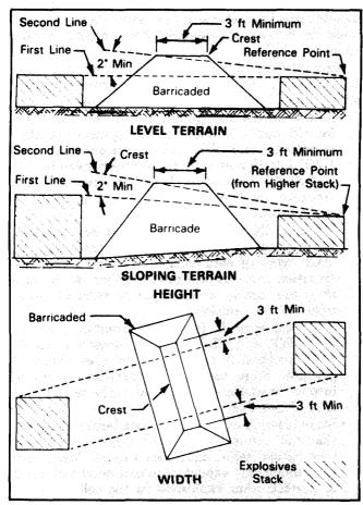
Figure 2-3. Barricade Dimensions Between Explosives Stacks.
