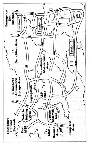
Figure 2-4. Typical ASP Layout.
