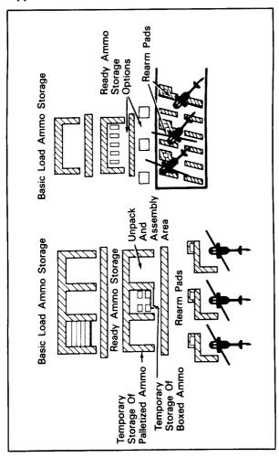
Figure B-1. Typical Layouts for Rearm Points.
